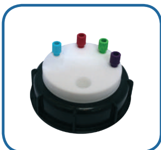
SW90-4-C : 4 entries 1/8" and a charcoal cartridge emplacement
