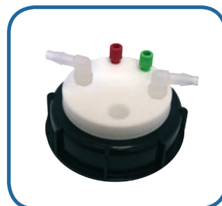
SW90-2-C-2L : 2 entries 1/8", a charcoal cartridge emplacement and 2 tube fittings
